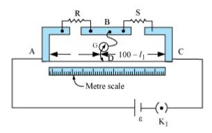
Here comma space R over S equals fraction numerator R subscript c m end subscript 1 over denominator R subscript c m end subscript left parenthesis 100 minus 1 subscript 1 right parenthesis end fraction therefore R equals fraction numerator S 1 subscript 1 over denominator 100 minus 1 subscript 1 end fraction
